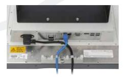
OPTIONAL: Cable protection / strain relief - connection side
