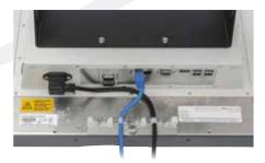
OPTIONAL: Cable protection / strain relief - connection side
